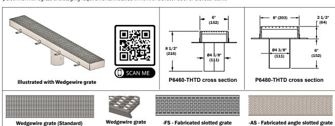
Note: The neoprene gasket used to connect long runs of trench drain channels is not recommended for use with caustic or harsh chemicals.
